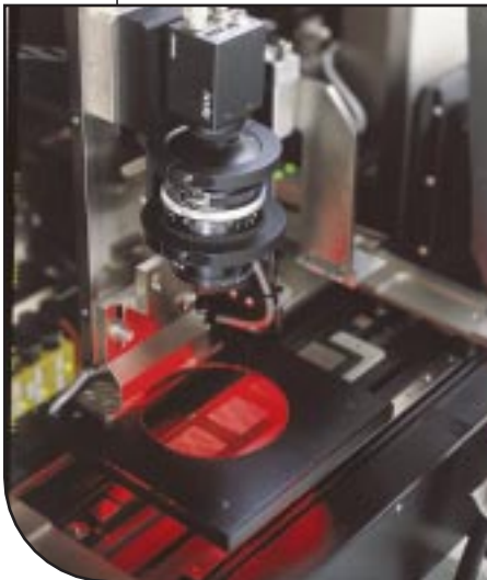
The PowerBGA system shown is integrated with an automated BGA sphere attach workcell conducting 100% inspection prior to the reflow process.
