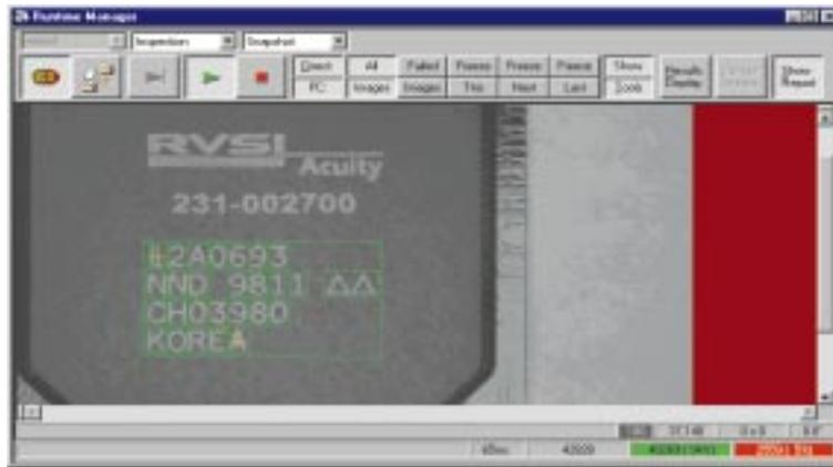
The Visionscape™ Mark Inspection system offers a built-in Windows® NT/95 Graphical User Interface (GUI) for point and click mark training, parameter setting and run-time inspection monitoring.
